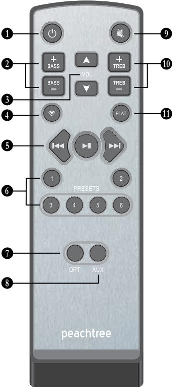
① **On/Standby Button:** With the AC power cord connected, this button toggles the unit between On mode (which selects the last input used) and Standby mode which lights the LED red. Note: the input LEDs will flash white in a sequence when the unit goes into on or standby mode.
